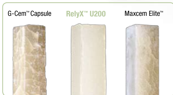
Results of stress test on self-adhesive resin cements. All samples were self-cured and thermocycled 10,000 times.
